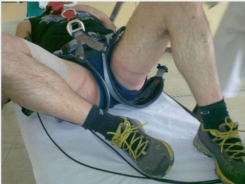
Figure 2: conditions of the teste after a inert suspension test of the duration of one hour. This photo shows the right position of the rescued person after the suspension.
